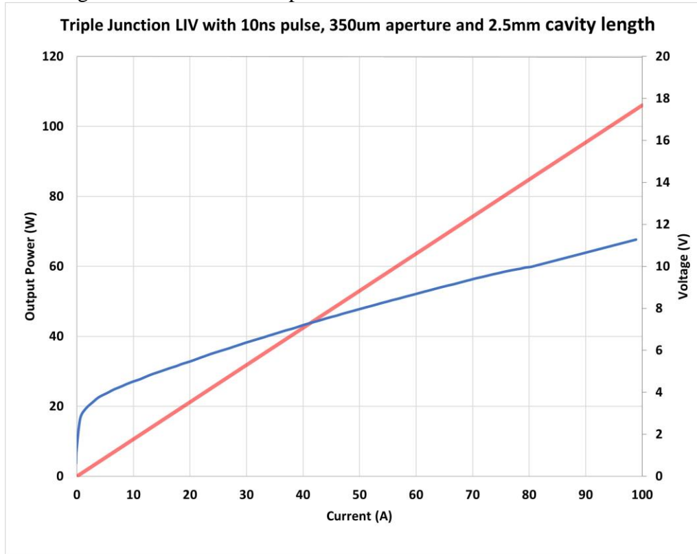
Fig.3 LI data of the new Triple Junction 1550nm laser diode of 10 nsec pulse
